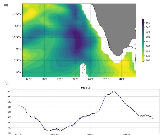
Fig 6. Difference between the depths of 20 degree and 10 degrees isotherms averaged for the month of November. b) The time series of the difference between D20 and D10 at 71E; 10N.
