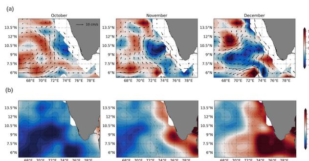
Fig 4. (a) The relative vorticity averaged for 200-400 m depth for the year 2003 from daily outputs of BLND overlaid by velocity vectors averaged for October, November and December months. (b) the lower panel shows the SLA from aviso during the same period.
